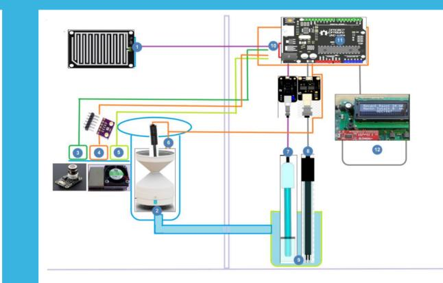
Automated module "RAIN-CONTROL". It is a small specialized meteorological station, created on the basis of the microcontroller ArduinoMicro and the set of the sensors. This device will allow automatic measurement of the main parameters characterizing atmospheric precipitation, namely:
